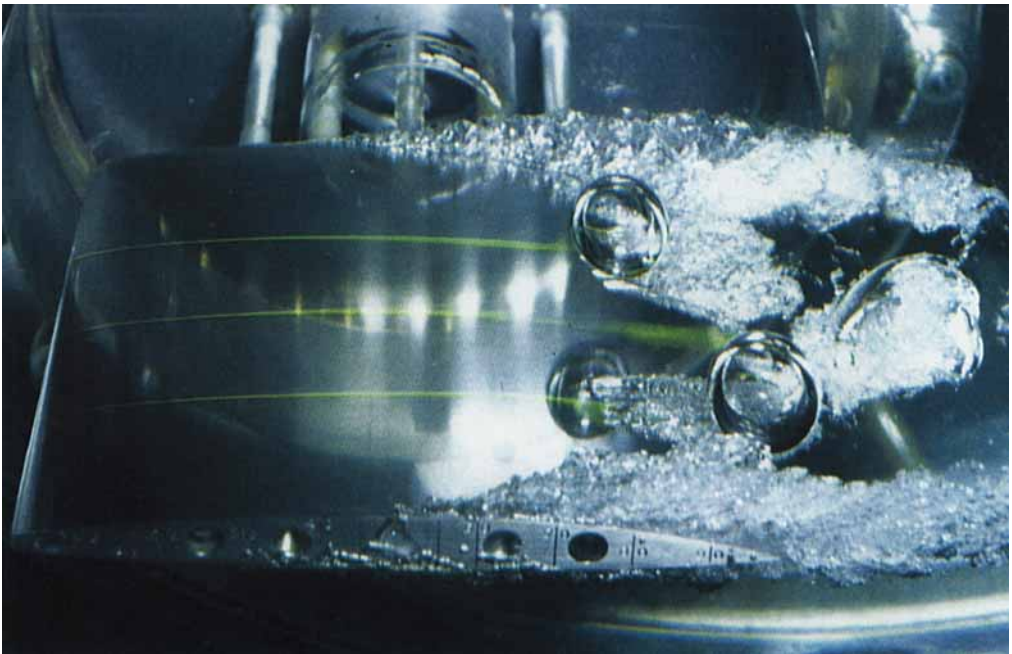
FIGURE 23. Sweeping away of a part of the rear cavity by a turbulent spot. Re=10^6 , \sigma_v=0.09 , \alpha=1^\circ .
